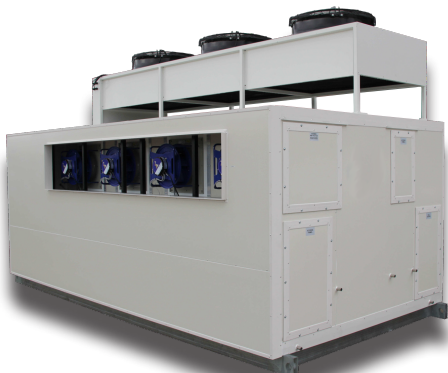
ACDHUM - outside air dehumidification with heat exchange precool and reheat to lower energy consumption. Available with DX or CHW cooling
