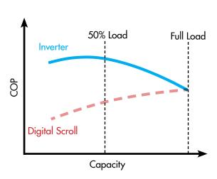
Indicative COP vs. capacity profiles of inverter and digital scroll compressors.
