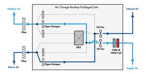
Used for free-cooling - when cold 100% outside air is brought straight into an indoor space to address the room load. Also used when the outside air temperature is mild and air-to-air heat / energy recovery is not necessary for supplying 100% fresh outside air.
