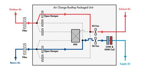
Used when 100% fresh outside air is not required (eg. when room occupancy levels are low). Outside air volume can be modulated between 0% and 100% to provide the minimum required fresh air and achieve further energy savings.
