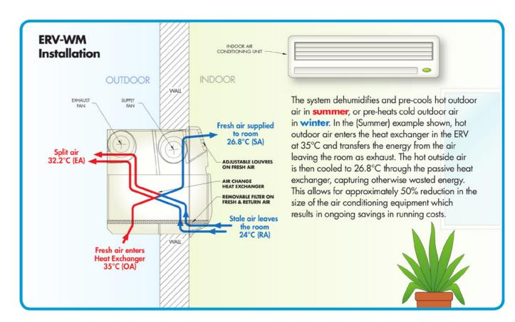
The ERV-WM unit can be located anywhere on an external wall or window of an air conditioned room, and is designed for a simple installation. Outdoor/Return air filter is accessible from inside the room.
