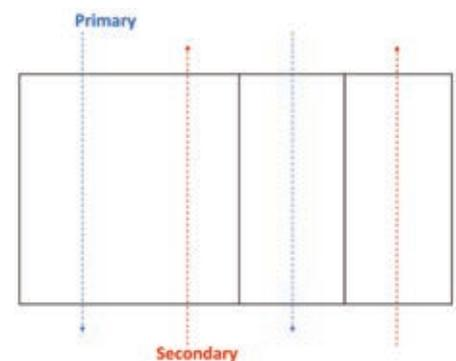
Figure 4 Counter Flow Heat Exchanger
