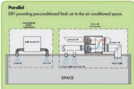
Figure 9 Ventilator in Parallel Operation
