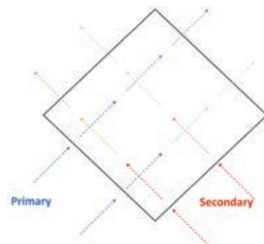
Figure 2 Cross Flow Heat Exchanger 2D
