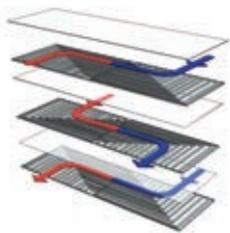
Figure 6 'Z' Flow Heat Exchanger 3D
