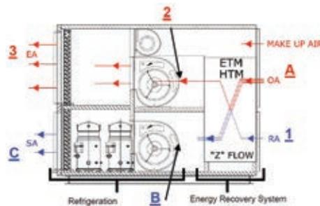
Figure 11 DX Packaged Unit with Heat Recovery
