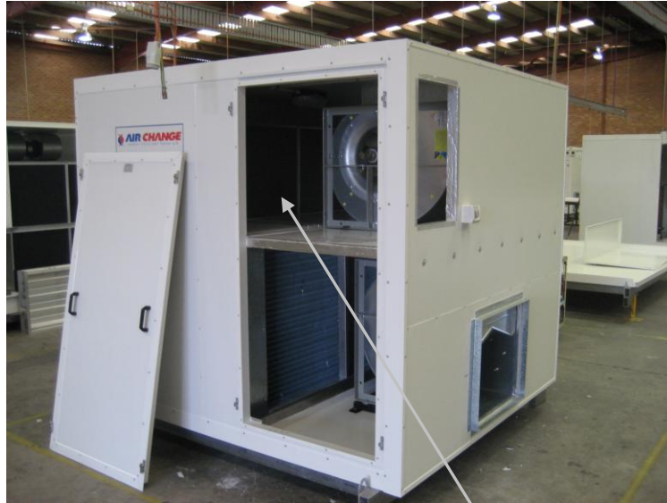
Access to Heat Exchanger face Internal
